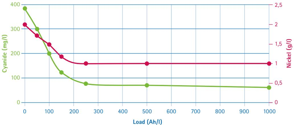
Image 8: Analysis progression of cyanide and nickel after conversion of the electrolyte in practice SLOTOLLOY ZN 210 VX.
