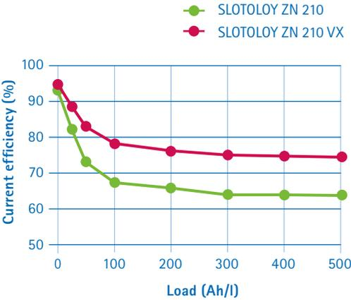
Image 3: Comparative current efficiency at  $i_k = 1 \text{ A/dm}^2$  (8 g/l Zn, 1 g/l Ni, 110 g/l NaOH)
