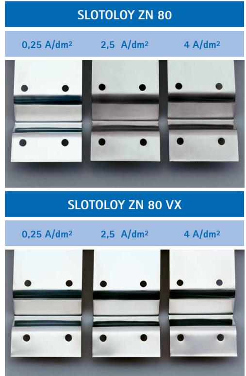
Image 4: Comparative lab panel series after an electrolyte load of 100 Ah/l.
