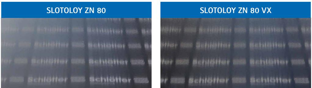
Image 5: Comparative Hull cell panels after an electrolyte load of 100 Ah/l. Electrolyte load, significantly brighter deposition when SLOTOLLOY ZN 80 VX is used.
